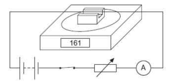
The balance, which was zeroed before the switch was closed, read 161 g after the switch was closed. When the current is reversed and doubled, what would be the new reading on the balance?
