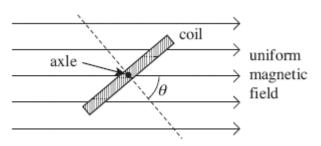
A coil of 50 turns has a cross-sectional area of  $4.2 \times 10^{-3}$  m<sup>2</sup>. It is placed at an angle to a uniform magnetic field of flux density  $2.8 \times 10^{-2}$  T, as shown in the diagram, so that angle  $\vartheta$  = 50°.
